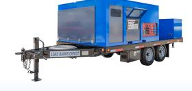
Larger capacity Load Bank specifically designed for direct mounting to DOT over the road trailer. Optional trailer shown here.
